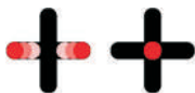
砲塔迴旋/Turret rotation: 第三動置中, 第四動撥桿向左或右撥 動,砲塔迴旋的速度與撥桿角度成正 比./Third moves sets, fourth moves the work driving arm towards left or moves right, the turret maneuver speed and the work driving arm angle are proportional.
